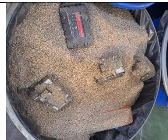
FIGURE 5. BATTERIES COVERED WITH VERMICULITE.
